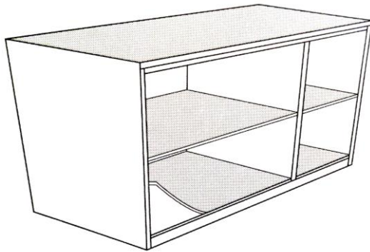
Framed/panelled (carcase) construction
